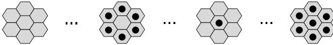
Fig. 2. Four of the possible 14 nearest neighbor configurations for TwoDOS. The dark circles in the cells depict a pit corresponding to a stored 1. Absence of a pit indicates a stored 0. In this case the pits cover only about half the area of the hexagonal bit cells. This is done to reduce signal folding [2].
