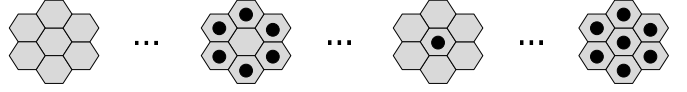
Fig. 1. Four of the possible 14 nearest neighbor configurations for TwoDOS. The dark circles in the cells depict a pit corresponding to a stored 1. Absence of a pit indicates a stored 0. The pits cover only about half the area of the hexagonal bit cells. This is done to reduce signal folding [8].
