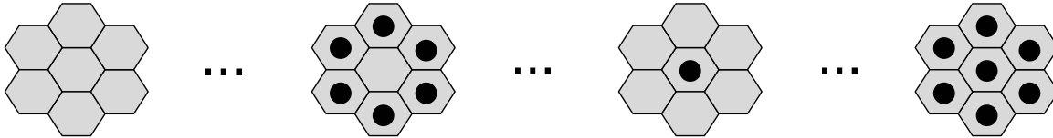
Fig. 1. Four of the possible 14 nearest neighbor configurations for TWODOS. The dark circles in the cells depict a pit corresponding to a stored 1. Absence of a pit indicates a stored 0. The pits cover only about half the area of the hexagonal bit cells. This is done to reduce signal folding [3].
