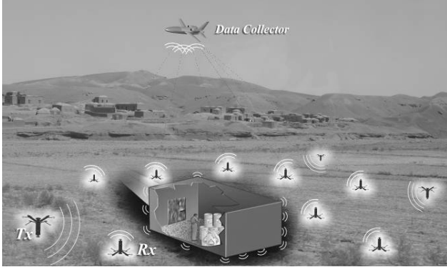
Figure 1: RF Tomography. Transmitters send power into the ground. Receivers collect the scattered field and send this information to the main station.
