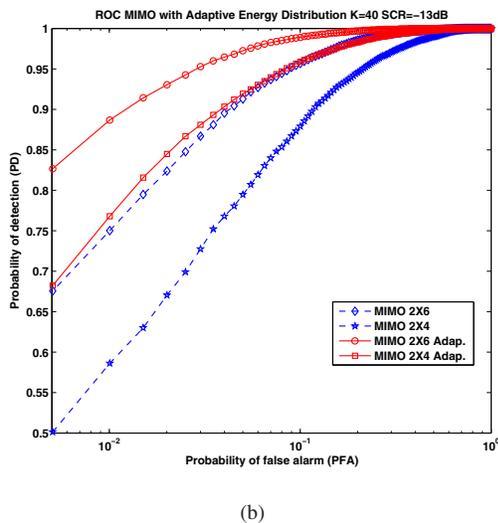
Fig. 2. (a) Receiver operating characteristics of MIMO and conventional phased-array radar (Conv.). (b) Receiver operating characteristics of MIMO radar with and without adaptive energy allocation.
